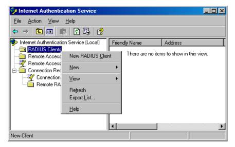
2. Enter a RADIUS client name (device name of the AP is recommended) and the IP address of the AP, and click **Next**.
